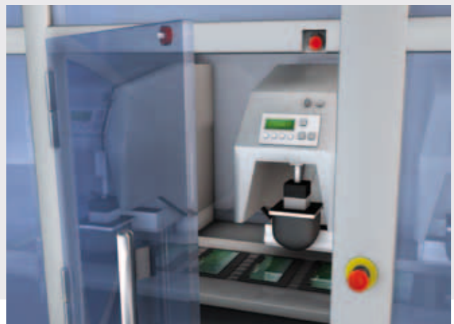
Cylindrical MC3x Sensor for guarding pad printing machines.
